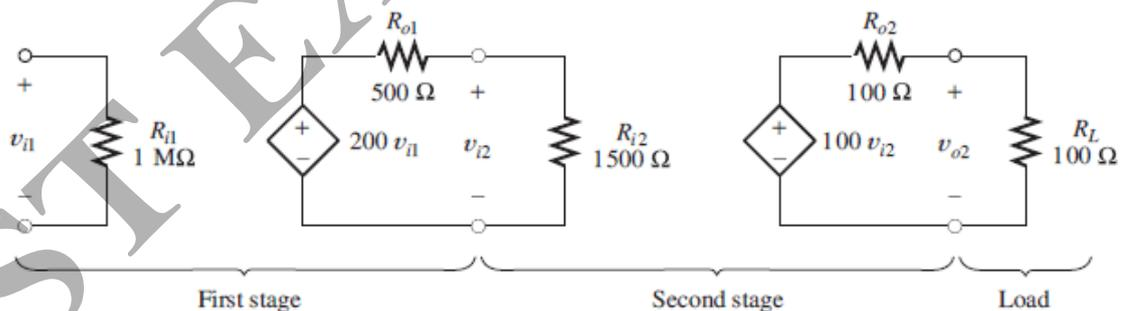
Fig.1(b): A cascaded amplifier circuit
