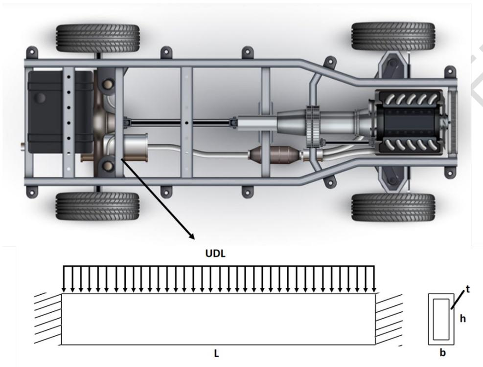
Figure Q6: Car Frame containing a clammed-clammed beam under UDL.
