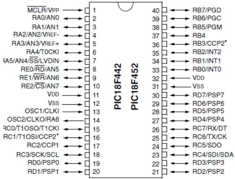
Figure 4: PIC18F452 Pinout
