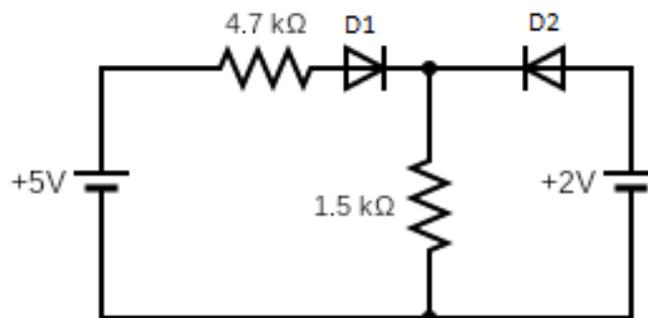
Fig.1(b) Diode circuit model
