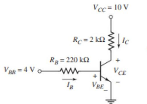
Fig.Q4(b): Transistor as an amplifier
