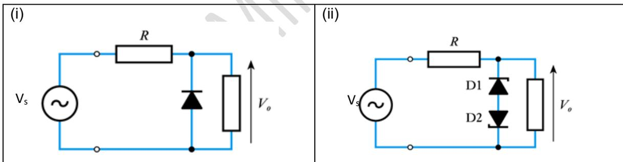
Fig.2(b). Diode circuits.
