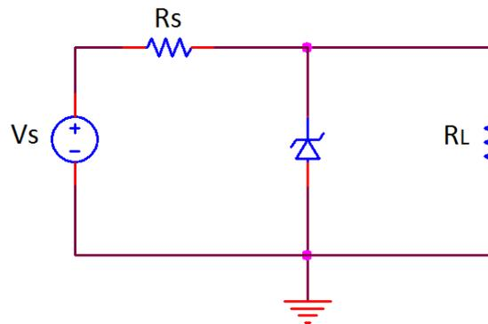
Fig.2(a). A voltage regulator circuit.
