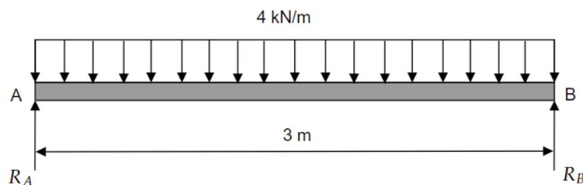
Figure Q6a: Simply supported beam with UDL.
