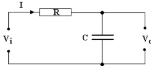
The voltage  $V_i = 10$  Volts. The charge of the capacitor in the circuit is described by the following 1st order differential equation:
