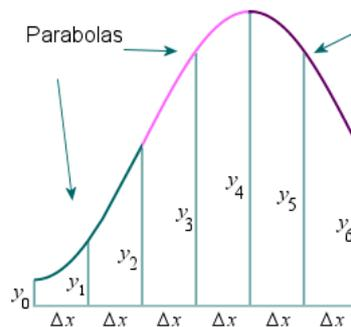
The area into  $n$  equal segments of width  $\Delta x$ . Note that in Simpson's Rule,  $n$  must be EVEN. The approximate area is given by the following rule:
